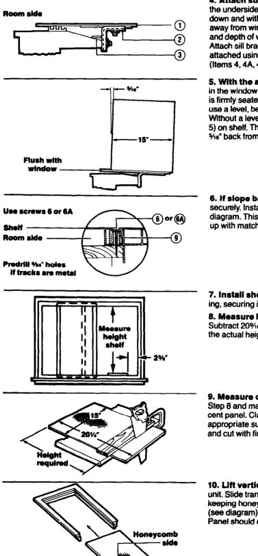
4. Attach support bracket (Item 2) loosely to the underside of shelf with either short or long leg down and with end of bracket either toward or away from window, depending upon construction and depth of wall and window sill (see diagram). Attach sill bracket (Item 3). Each bracket is attached using one 5/16'' bolt, nut and washers (Items 4, 4A, 4B and 4C).
